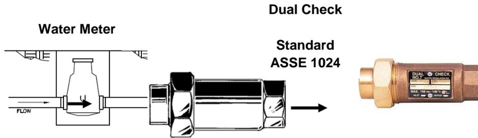
**Description (DuC).** A dual check shall contain two internally loaded, independently operating check valves. A dual check shall be a device approved by an approval agency acceptable to the local administrative authority.
